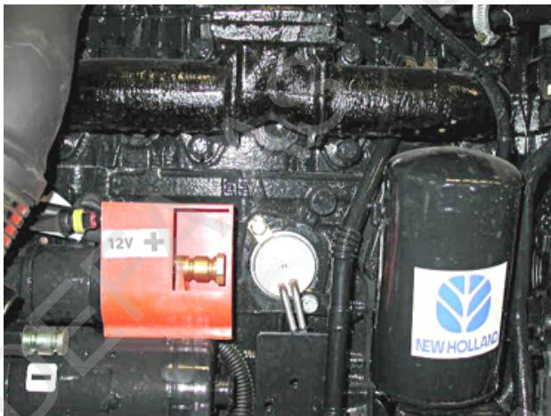
GB Fit the heater from underneath. Remove the frost plug (1). **Note!** Thoroughly clean the hole for paint and corrosion. Dismount the fastening bolt (2) for the coolant pipe. Fit the heater, using the supplied fastening brackets and screws with lock washers (3). Ensure that the brackets are correctly placed on the flange of the heater. Fit back the fastening bolt (2) for the coolant pipe. Top up with coolant and bleed the system, as specified by the car manufacturer. Check for leaks.
